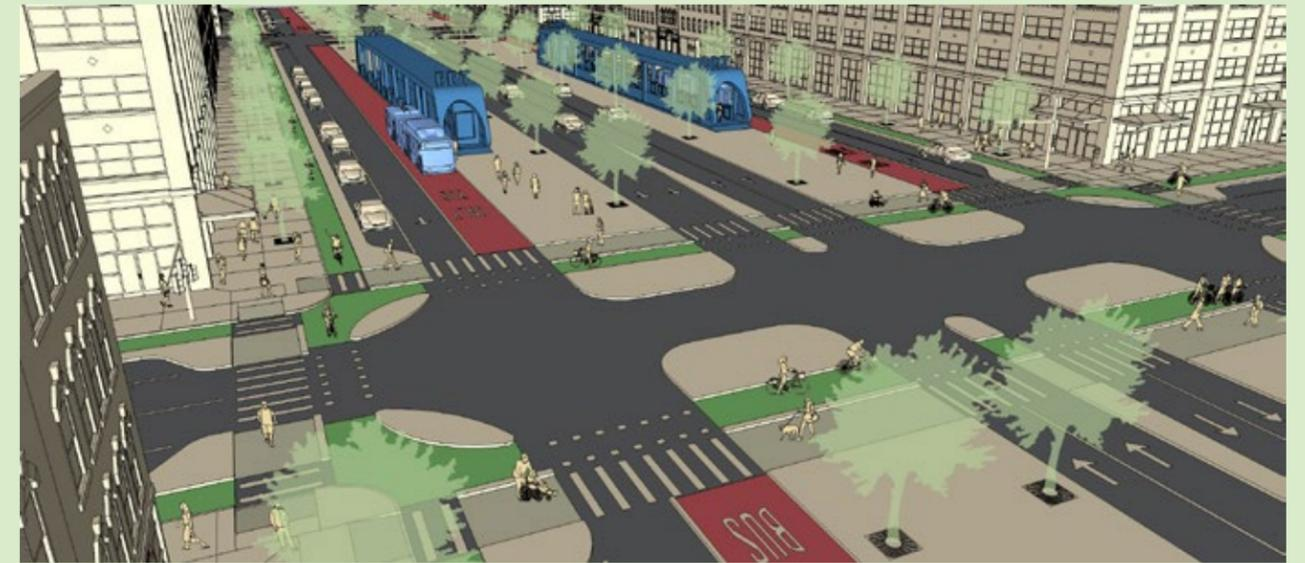
**EXAMPLE OF A BUSWAY ALIGNED TO THE INNER CURB OF THE SERVICE ROAD ON A BOULEVARD-TYPE STREET WITH A CENTRAL ROADWAY AND PARALLEL SERVICE ROAD**
