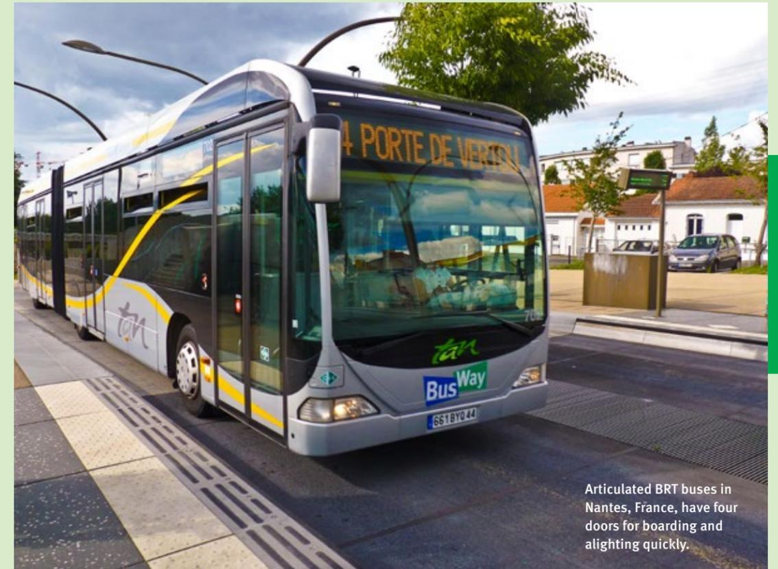
Articulated BRT buses in Nantes, France, have four doors for boarding and alighting quickly.
