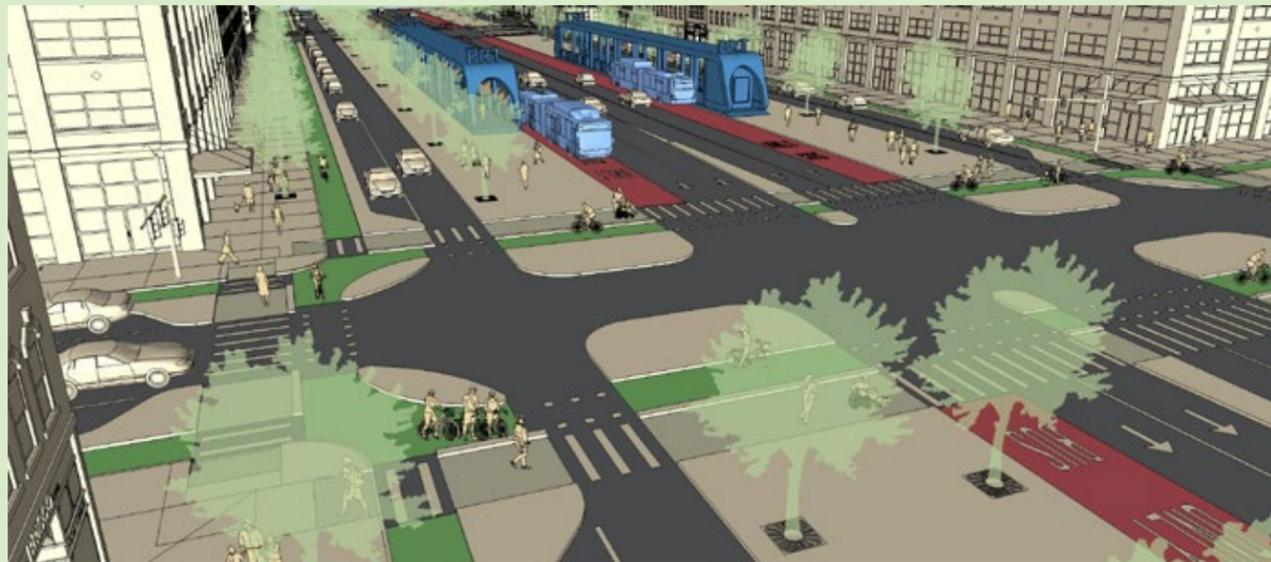
**EXAMPLE OF A BUSWAY ALIGNED TO THE OUTER CURB OF THE CENTRAL ROADWAY ON A BOULEVARD-TYPE STREET WITH A CENTRAL ROADWAY AND PARALLEL SERVICE ROAD**
