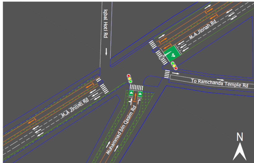
Figure 7.21 Proposed Junction Design for M.A. Jinnah Rd - M. bin Qasim Rd Junction
