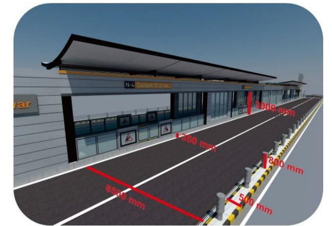
Station Exterior Dimension
