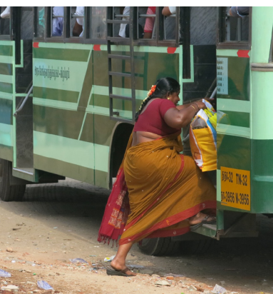
Bus stops without platforms for level boarding and vehicles with big steps make getting on and off the bus stressful and cumbersome especially when carrying goods or young children. Tiruchirappalli, India. Source: ITDP.
