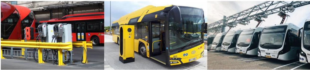
Figure 3. Types of charging equipment positioning: docking station, free-standing, overhead
