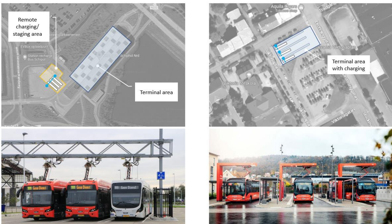
Figure 20. Above left, Amsterdam remote charging and above right, Jönköping 'rank' style on stand charging
