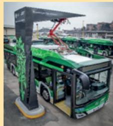
Gambar 2. *Inverted pantograph*<sup>21</sup>
