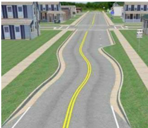
Figure 6. Chicane (Left) and Textured Street (Right)
