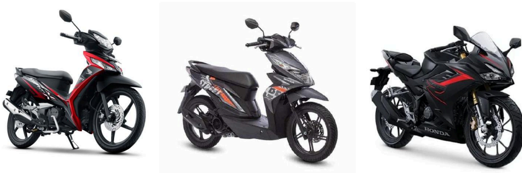
Figure 5. Motorized 2W Body Types From left to right: Underbone, Scooter, and Motorcycle (source: astra-honda.com )
