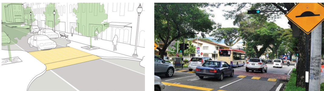
Gambar 3.28. Penerapan Speed Table (sumber: NACTO Urban Street Design Guide and penangmonthly.com , 2013)
